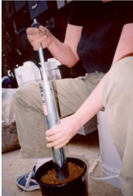
Figure 2. Compaction of soil in nursery pots using a standard compaction hammer.
