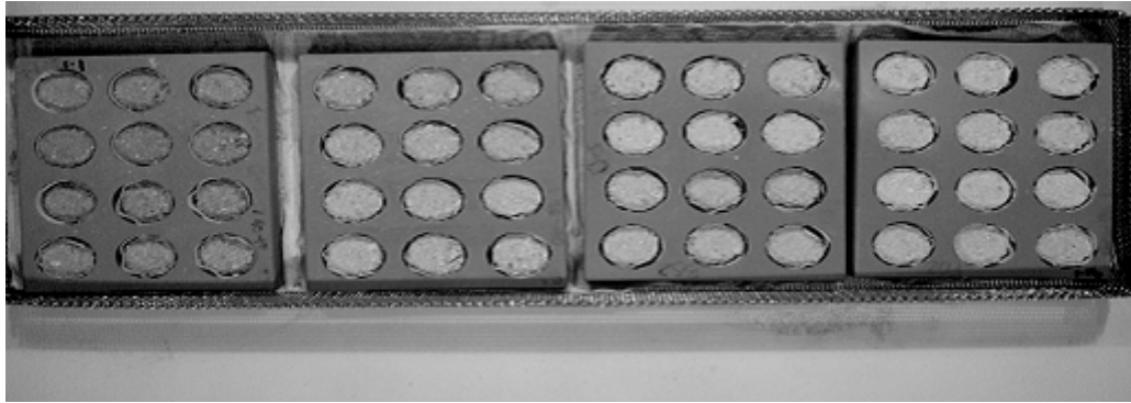
Figure 1: Four modulus of rupture trays with each circle representing the area used for Image J analysis.
