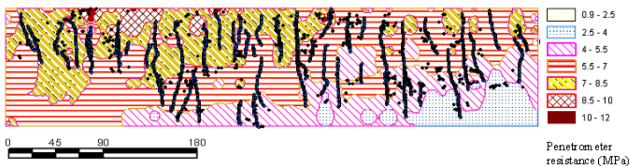
Figure 3. Inverse Distance Weighted map of penetrometer resistance with cracks and roots along a profile wall (T5)(TGR) (20 cm grid; 259 locations).
