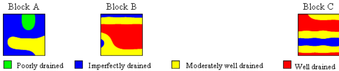
Figure 3 .Soil drainage class maps for the 300m by 250m window (7.5 ha) areas when mapped at 1:10,000 scale.
