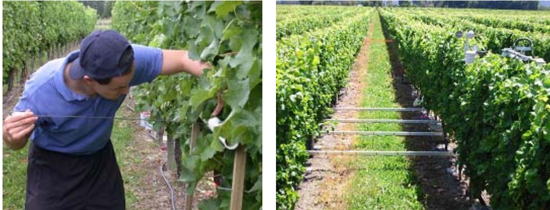
Figure 1. The left hand panel shows point-quadrat measurements of leaf area being taken at the Squire Estate. The right hand panel shows an array of light sensors used to measure light interception and to deduce a 'crop factor'.
