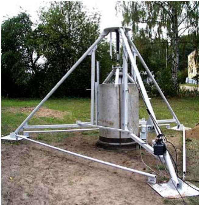
Figure 1. Cutting tool for obtaining large undisturbed soil monoliths.
